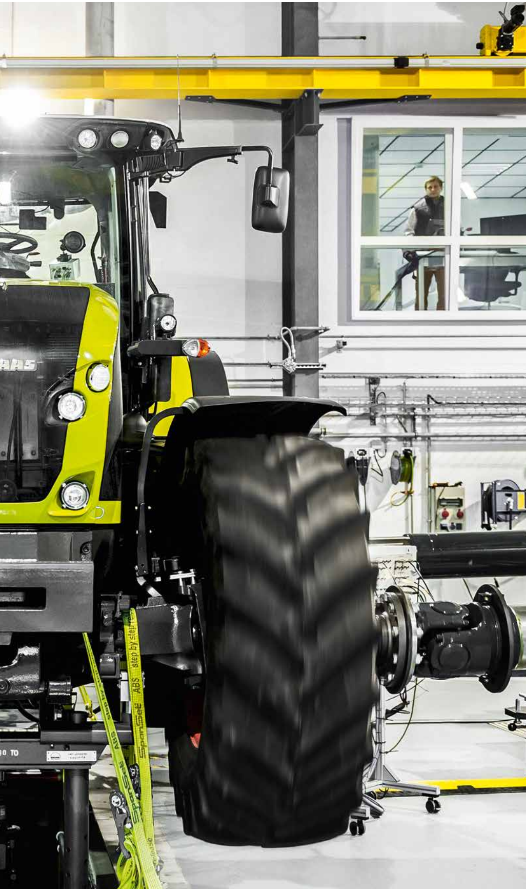
1 Moving without motion: a tractor on the drive test bench in Trangé.
